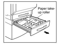
2 Press down on the paper-lifting plate until it locks into place.
